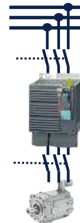
Drive system with external motor and line contactor
