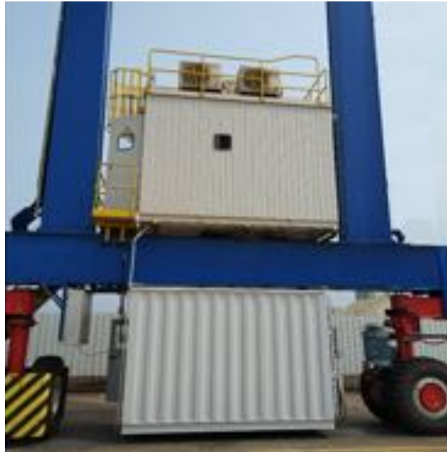
Battery housing mounted under sill beam
