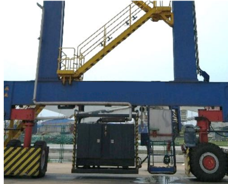
Small diesel genset mounted under sill beam
