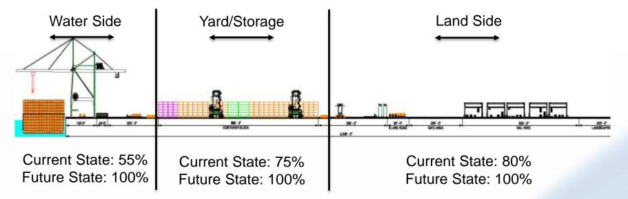
Container handling solutions for horizontal transport should be prioritized, since it has the greatest impact on throughput. The **stack is the main** problem - its low service levels is the main reason contributing to the other container 'handling' processes.
