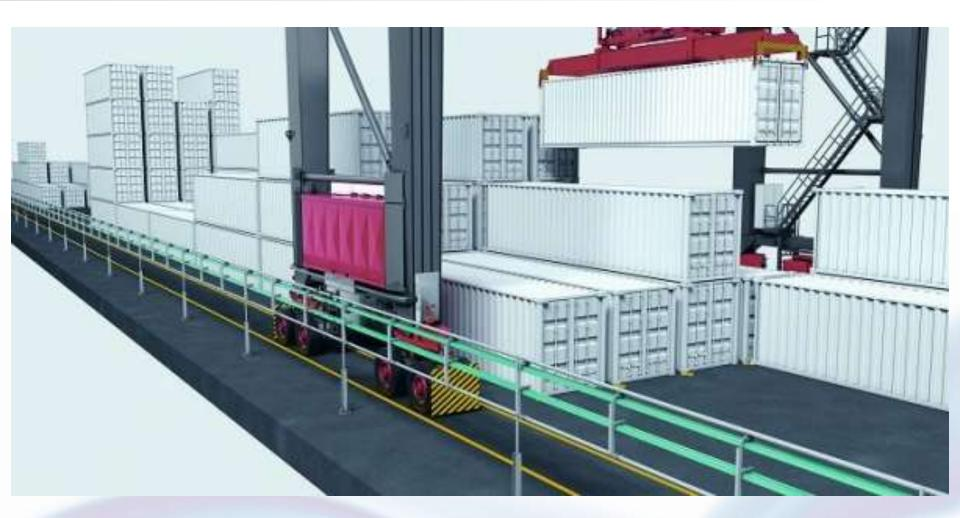
The Busbar power connection converts the RTGs to fully electric operation. **Image: Konecranes**
